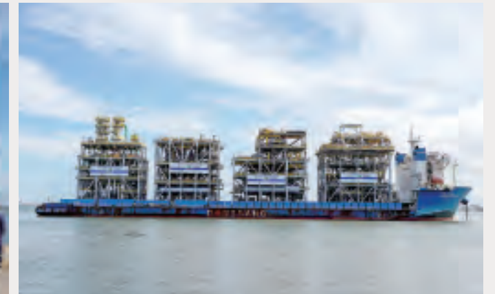
Four modules being shipped to the integration yard
