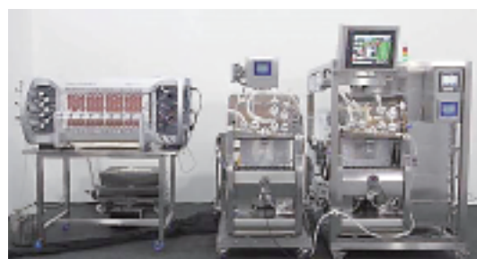
Left: Pall Corporation's continuous chromatography unit Right: TPS's continuous virus inactivation unit
