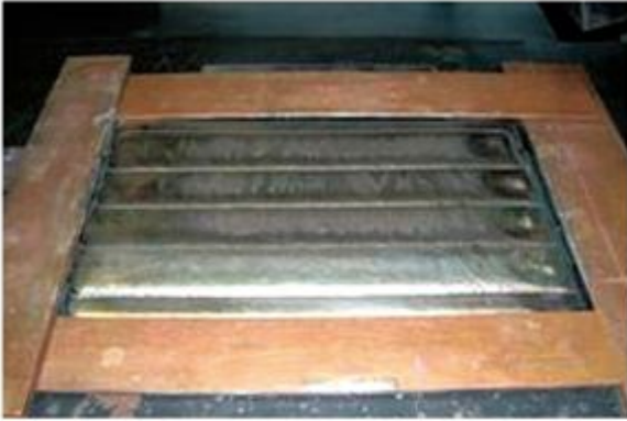
Fig. Appearance of weld overlay by ESW. Matching filler metals have been developed for gas tungsten arc welding (GTAW) and electro slag welding (ESW). No undercut is observed at fusion boundary.
