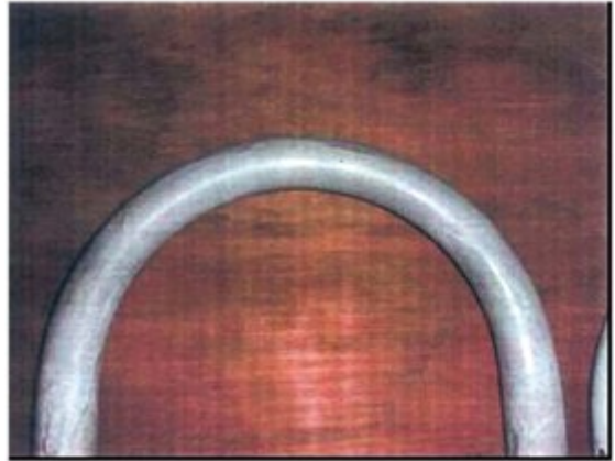
Fig. Appearance of bended U tube of DP28W. DP28W™ has good formability. Flaring and flattening test is also satisfied.
